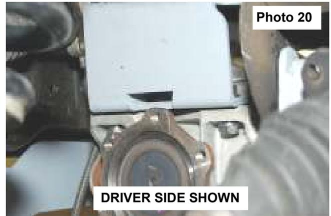
30. Tighten the diff drop brackets (65ft. lbs) to the frame and the differential to the diff drop brackets using a 18mm wrench .
