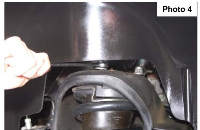
8. Using a 15mm wrench, remove the 2 bolts securing the lower strut mount to the lower control arm and remove the strut from the vehicle. Remove and discard the factory lower retainer clips. New hardware will be used. **See Photo 5**.
