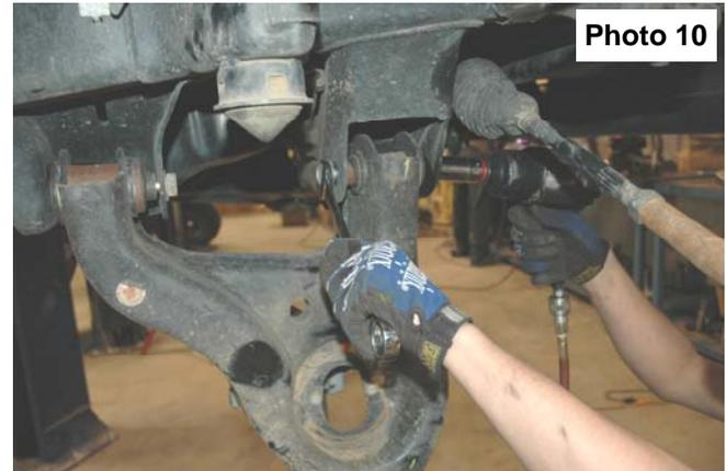
17. Hang the new Rough Country front cross member in place. Use factory hardware from lower control arms to bolt in place, do not tighten at this time.
