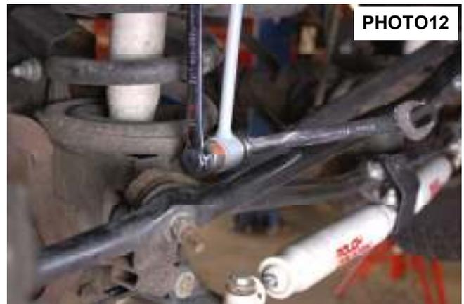
29. Raise the front axle with a floor jack to slightly compress the coil springs.
