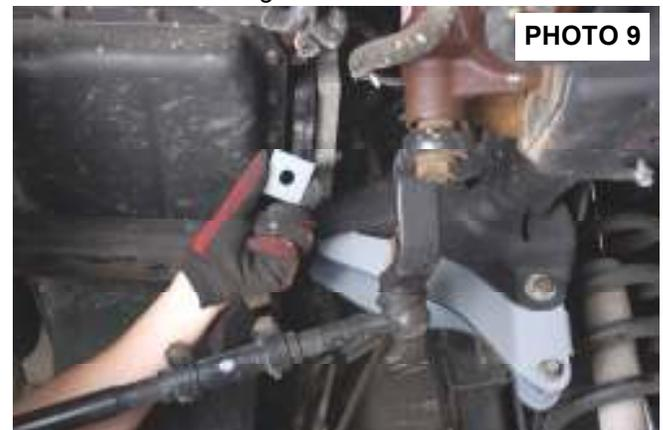
25. Install the new pitman arm into the stock location on the sector shaft, using stock hardware and torque nut to 185 ft. lbs. **See PHOTO 9.**
