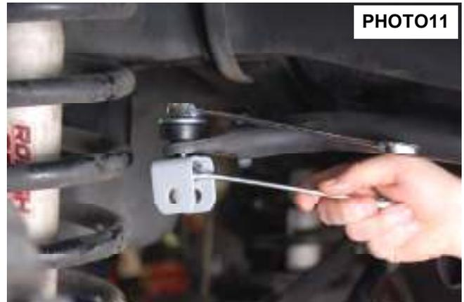
28. Install the supplied bushings / sleeves in the new sway bar links and install in the new sway bar bracket as shown **PHOTO 11** and on the factory axle location with supplied 12mm x 65mm hardware. **See PHOTO 12.** Tighten hardware.
