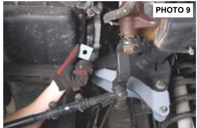
23. Install the new pitman arm into the stock location on the sector shaft, using stock hardware and torque nut to 185 ft. lbs. **See Photo 8.**
