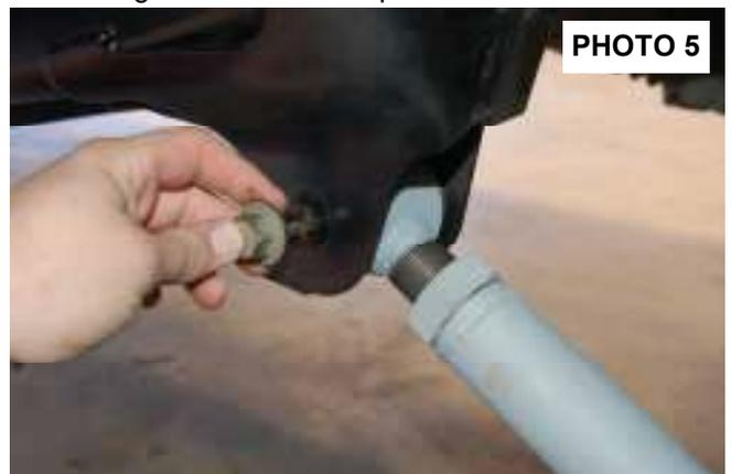
14. Remove the upper suspension arm nut and bolt at the axle. Remove the nut and bolt at the frame and remove the upper suspension arm. Repeat this step for the opposite side of the vehicle. **Note: If your truck has a diesel engine it may be necessary to unbolt the exhaust from the turbo to allow for clearance to remove the upper front bolt.** Retain hardware for reuse.
