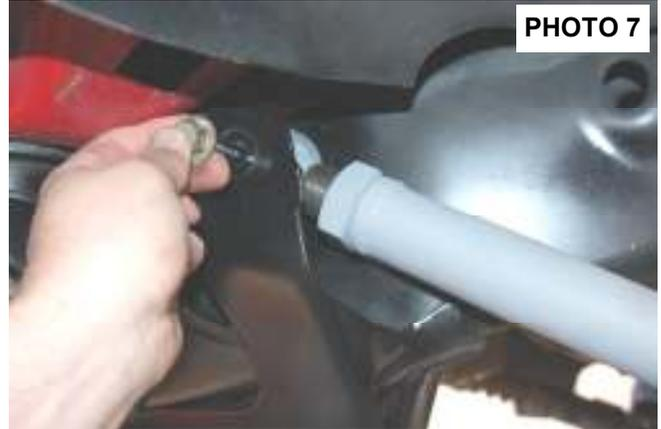
17. Remove the lower shock bolts on the axle, and save for later installation. The shock absorbers will be removed from the vehicle at the same time the coils are removed from the vehicle.
