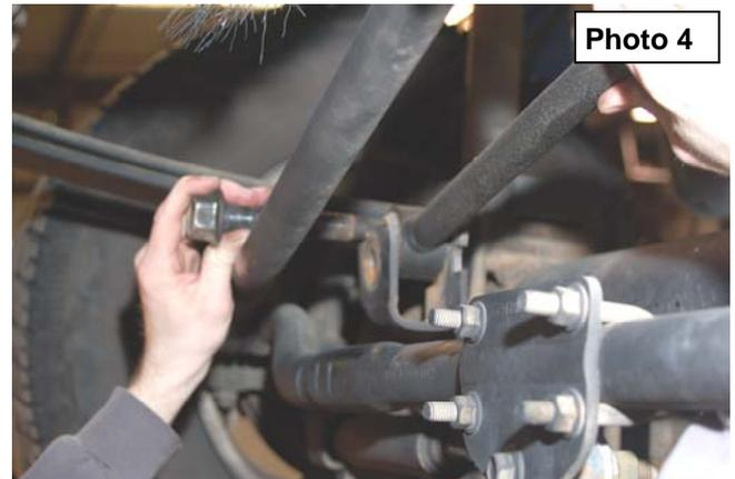
4. Remove the front shock absorbers from the upper mount and the lower mount from the axle using a 19mm wrench . Retain the hardware for re-use. Remove the shock absorber.
