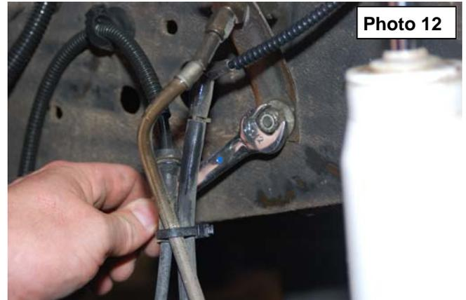
25. Install the new brake line on the caliper with factory hardware.
