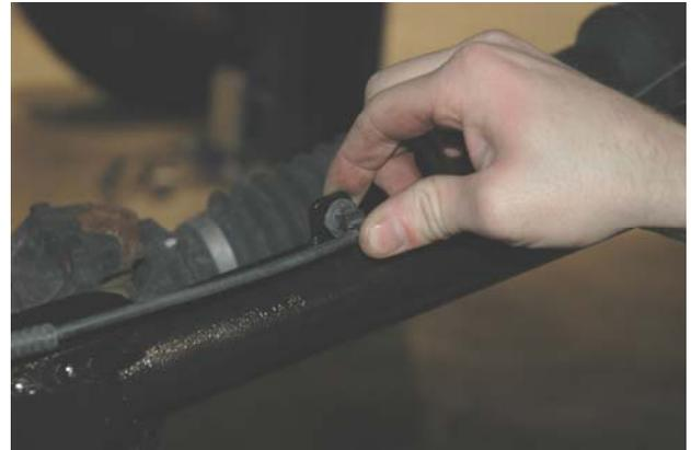
18. Using a 21mm wrench and 18mm wrench socket remove the factory track bar bracket. Retain stock hardware for re-use.
