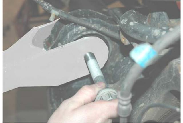
14. Attach the lower control arm to the axle using the stock hardware. Do not tighten at this time.
