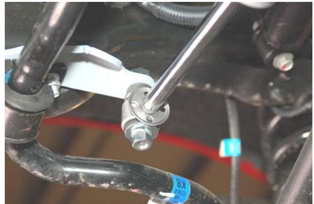
29. On the driver side, remove the sway bar bracket from the frame using a 15mm wrench and install the supplied spacer plate as shown in **Photo 11** with factory hardware.
