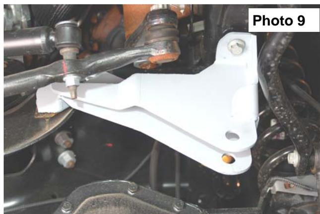
18. Using the nylon bump stop extension provided, place the extension between the frame and the bump stop cup. Bolt back into the original location using the 8mmx95mm bolt supplied. Torque to 15 ft. lbs.
