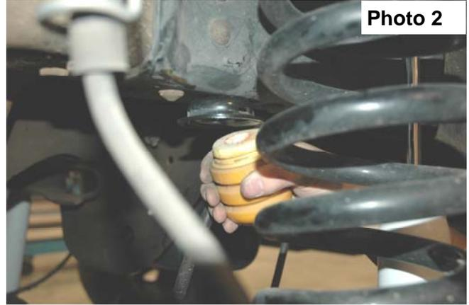
5. Disconnect the ABS sensor wire from the lower spring seat and the radius arm, using a 8mm wrench.
