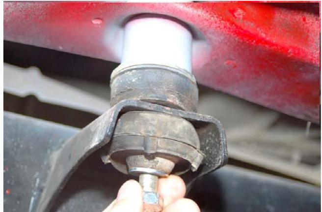
5. Insert the supplied body lift blocks in the 4 rear most mounts. Apply thread locker to the supplied 7/16" x 4" bolts and install. **Photo 3** shows all body mounts. Rear corner mount shown in **Photo 4**. Do not tighten at this time.
