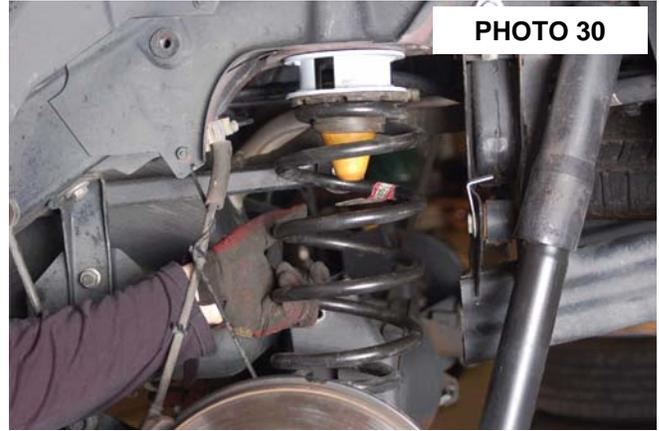
11. If removed, reinstall the upper control arm bolt at this time using a 18mm socket. Raising or lowering the floor jack may be needed to align the control arm to the mount.
