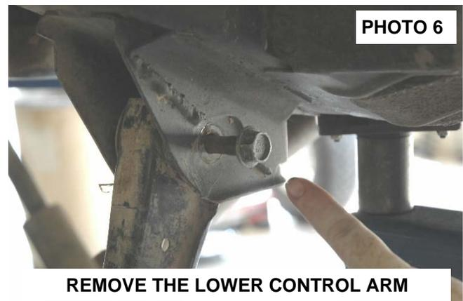
11. Insert the supplied bushings and sleeves in the lower control arm, lightly apply grease to bushings and sleeves. Adjust the arm to 16 1/2". The straight male end goes to the frame mount, offset end mounts up on the axle. Using a 21mm socket and 18mm wrench install the lower control arm in the axle mount. Using a 21mm wrench and socket install the control arms in the frame mount, using stock hardware. Do not tighten at this time. **See PHOTO 7 & 8.**
