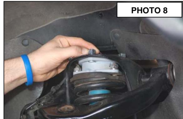
11. Position the strut assembly to reinstall the lower strut bolt in its original position that it was removed. Using original hardware and a 19mm socket torque to 100ft lbs.
