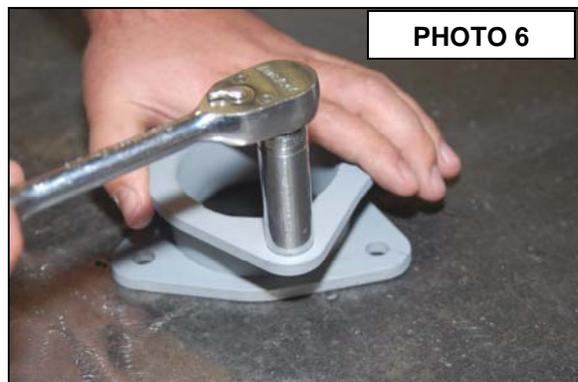
9. Install the new spacer with the studs pressed in on the strut assembly and install the spacer on the strut assembly with the stock hardware. **See PHOTO 7.**
