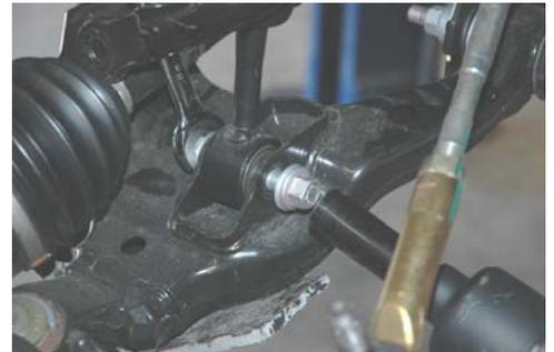
9. Locate the supplied 3/8" stud extensions. Using a 9/16" socket snug self clinching stud in the new spacer as shown in **Photo 7.** **The stud should clinch with about 35-45 ft/lbs of torque. Do not over torque the nut.**
