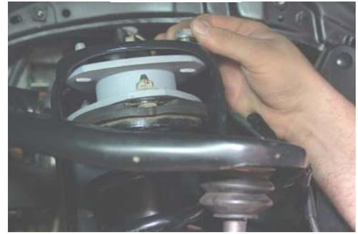
12. Position the strut assembly to reinstall the lower strut bolt in its original position that it was removed. Using original hardware and a 19mm socket torque to 100ft lbs.
