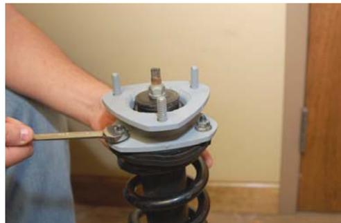
11. Install the strut assembly into the strut tower and start the supplied 3/8" nuts. Using a 9/16" wrench torque to 47ft. lbs **See Photo 9.**
