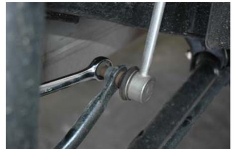
5. Using a 12mm wrench remove the bolt holding the brake line bracket to the frame on the drivers side, and the ABS wire on the passengers side.
