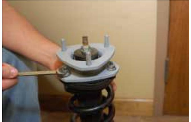
11. Install the strut assembly into the strut tower and start the supplied 3/8" nuts. Using a 9/16" wrench torque to 47ft. lbs **See Photo 9.**
