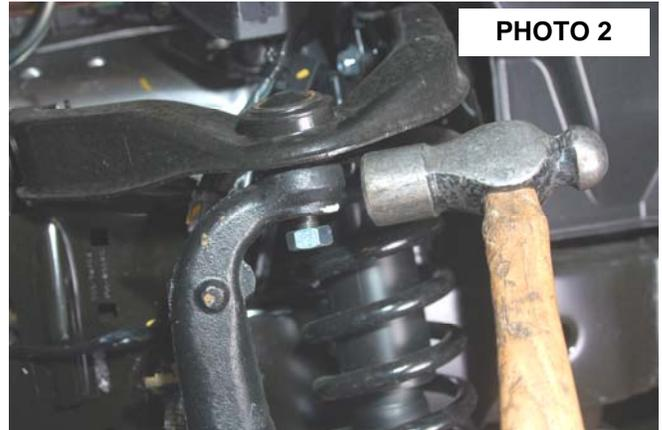
3. Remove the upper ball joint cotter pin and the upper ball joint nut using a 22mm wrench. Hit knuckle as shown to release the upper ball joint, **See PHOTO 1 & 2.**
