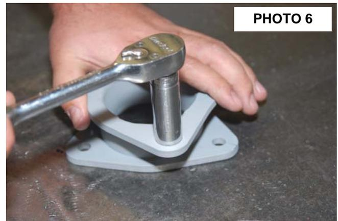
9. Install the new spacer on the strut assembly as shown in **PHOTO 7** with factory hardware and using a 14mm wrench.
