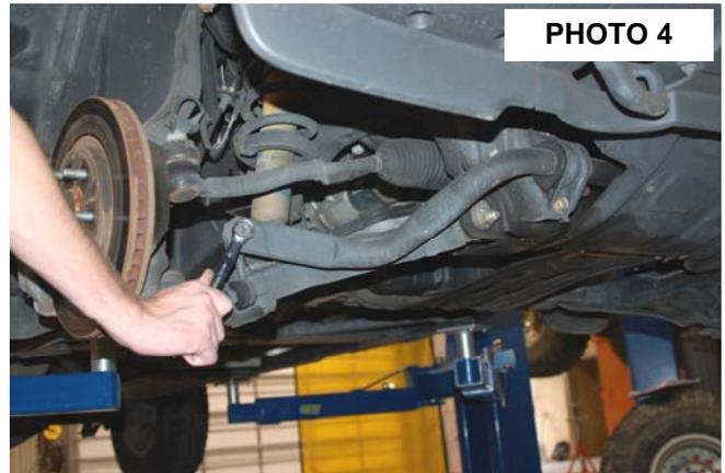
5. Remove the sway bar from the sway bar link using a 17mm wrench. **See PHOTO 4.**
