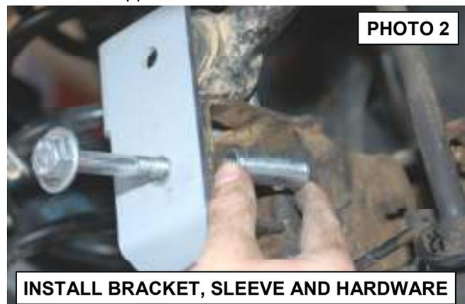
5. Using the bracket hole as a guide and using a 5/16" drill bit, enlarge the 2 holes in the axle mount to accommodate the 5/16" x 1" bolts.
