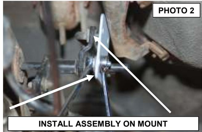
4. Install the supplied drop bracket on the stock tunnel bracket with the supplied 1/4" x 3/4" bolts/washers & nuts. Tighten hardware using a 7/16" wrench. Check clearance on bolts. **See Photo 3 & 4.** In Photo 3, bracket is shown removed to show mounting location. It is not necessary to remove the bracket although it can be removed to ease installation.
