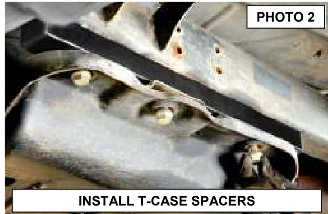
**Note:** If your vehicle is equipped with a 4 speed automatic and is a 2003-2006 you will have an additional cross member connected to the transfer case by a plate. On this vehicle a total of 2 spacers are used per side. In situations where you are using this vehicle with the front sway bars disconnected (and during full droop during installation) the front drive shaft may hit this cross member.
