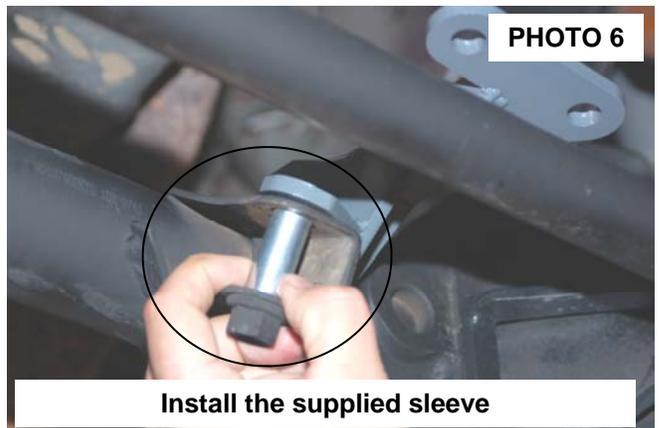
7. Using the thick wall sleeve 3/8" I.D x 1.400 long in the poly bag, insert this sleeve into the rod end of one of the stabilizer cylinders. This cylinder will be used on the passenger side.
