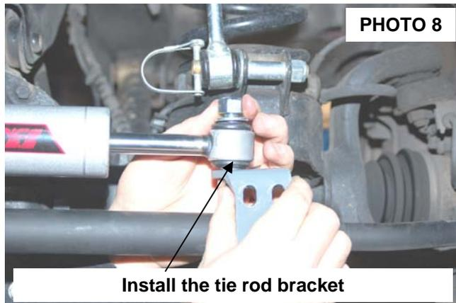
11. Next using the 2- 3/8" x 1 1/2" u-bolts and 3/8" flange nuts, install the tie rod bracket to the drag link. Extend the stabilizer 1/4" from fully extended and tighten the 3/8" flange nuts with a 9/16" socket. **See Photo 9.**
