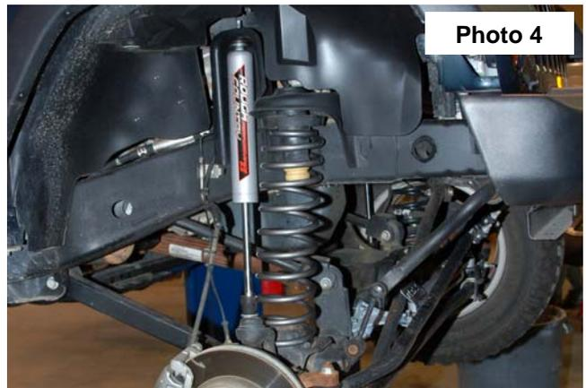
10. The draglink must be adjusted to center the steering wheel **BEFORE** the vehicle is driven. Failure to do so will cause a computer error with the Jeep's traction control system and will result in odd handling and poor performance.
