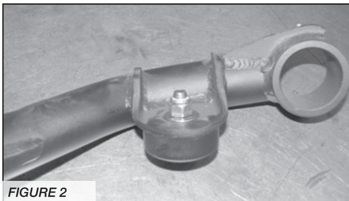
7. Install the new Fabtech upper control arm in the factory upper control arm pockets using the factory hardware at the previously marked alignment cam location. When installing the arm on the truck make sure the barrel gussets are up. Torque to 150 ft- lbs.
