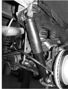
11. Reinstall the factory shocks onto the lower axle mounts and the new dropped upper mount using the original hardware.
