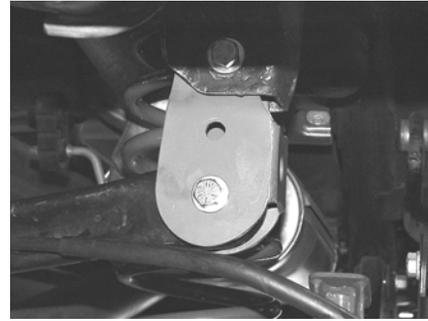
13. Raise the floor jack supporting the rear axle and slide the upper mount of the track bar into the drop bracket. Align the track bar with the lower hole and reinstall the factory bolt.
