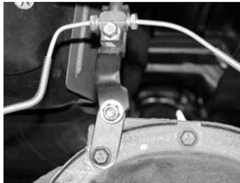
12. Connect the bottom of the sway bar end link onto the sway bar using the supplied 12mm-1.75 x 70 bolts, flat washers and nylock nuts. Install the brake line extension tab using the original bolt and the supplied 5/16" grade 5 hardware.
