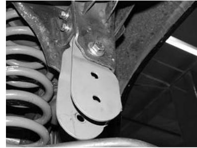
7. Slide the track bar drop bracket into the original frame mount. Place the supplied 9/16" bolt, with a flat washer, through the original hole, followed by another flat washer and a nylock nut. Do not fully tighten. Place 5/16" lock washers followed by 5/16" flat washers on both 5/16" x 1" grade 8 bolts and thread them through the existing holes in the frame mount and into the nuts on the drop bracket. Tighten the 5/16" bolts to 15 ft./lbs. Followed by the 9/16" bolt to 75 ft./lbs.
