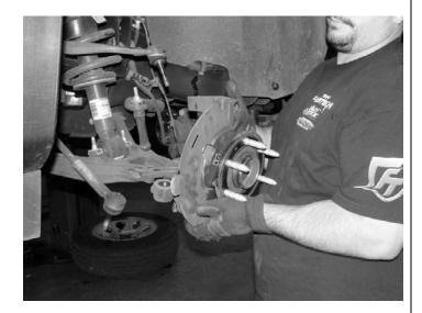
5. Drill out the top tapper on the factory spindle to 34". This is to allow for the 34" bolt to pass through the spindle.
