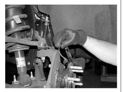
4. Remove the nuts securing the tie rod, upper and lower ball joints to the spindle. Separate all three joints from the spindle and remove the spindle from the control arms. SEE PHOTO BELOW
