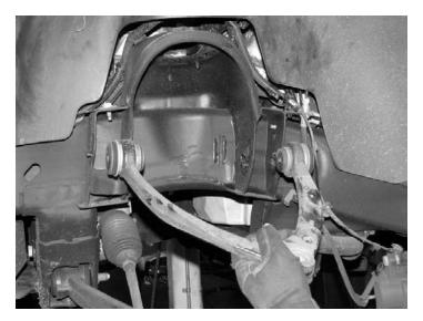
Using a die grinder remove the factory droop stop off the control arm pocket.
