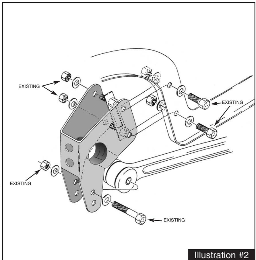
6. Remove the stock coil springs from both the driver and passenger side of vehicle. Unbolt the stock radius arms, remove the original radius arm frame brackets and remove from front axle housings.
