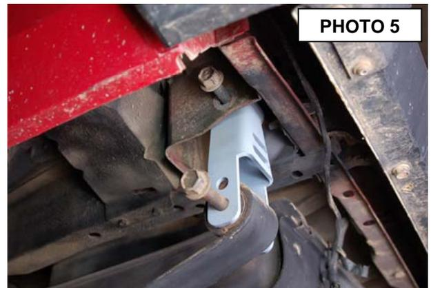
3. Install the new shocks with factory hardware. Torque the upper using a 13mm wrench and lower bolts using 3/4" wrench to factory specs. Repeat for other side.
