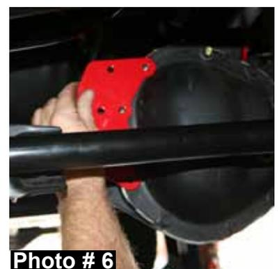
12. Attach the new Skyjacker track bar differential bracket (D30 or D44) to the differential using the supplied 5/16" x 1" bolts. **Note:** Do not tighten at this time. Install the new Skyjacker brace between the third member & track bar bracket. **Note:** Be sure to use the thick, gold plated 5/16" washer between the bracket & the differential cover. Use the 5/16" lock washer under the head of each bolt. (See Photo # 7) **Note:** Do not tighten at this time.
