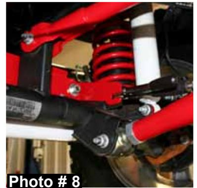
14. Drill a 7/16" hole through the new brace into the spring perch & install the supplied 7/16" x 1" bolt, washer, & nut to the perch. Tighten at this time.
