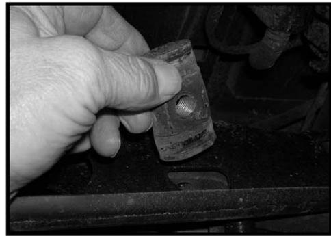
5. Working on the driver side, tap the torsion bar forward until the torsion bar key can be removed. Remove and discard the torsion bar key.
