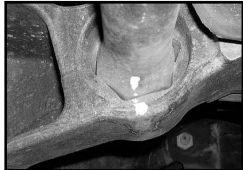
7. Using the torsion bar unloading tool, adjust the new torsion bar key up high enough so that the torsion bar block and bolt can be re-installed.
