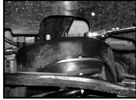
14. Locate the stock lower strut hardware. Secure the lower portion of the stock strut into the stock location using the stock hardware. **Special note: Make sure to use thread locker or loctite and torque to 65 ft lbs.**
