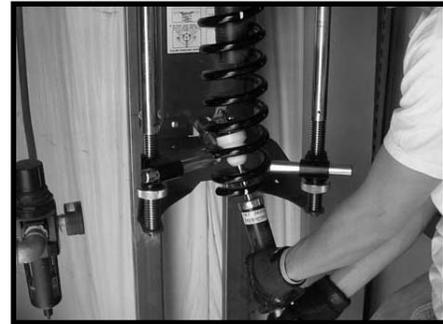
9. Working on the driver side upper bearing plate, remove the stock dust boot and discard. Place the isolator aside.
