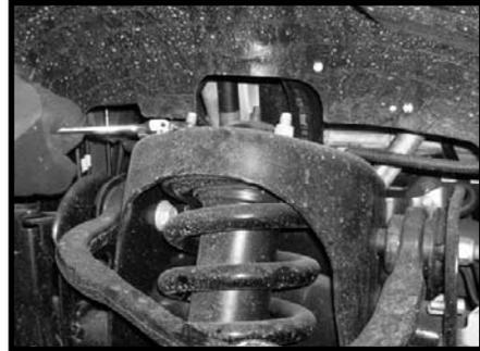
4. Working on the driver side, remove the stock lower bolt that connects the lower stock mounting point to the stock lower strut. Set the stock lower bolt aside for later re-installation. Repeat procedure on the passenger side.
