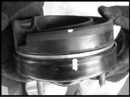
12. Compress the stock strut enough so that the new front spacer can be installed. Install the new front spacer and secure the stock strut assembly with the stock upper hardware. Refer to the reference marks and make sure that they line up. **Special note: Make sure to use thread locker or loctite and torque to 45 ft lbs.**
