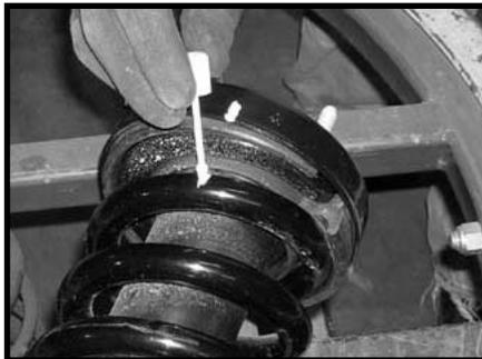
Tuff Country EZ-Ride Suspension highly recommends using a wall mounted strut compressor when installing the strut spacer into the stock strut. If you do not have access to a wall mounted strut compressor, please take it to your local Ford dealer to have the strut spacer installed into the stock strut.
