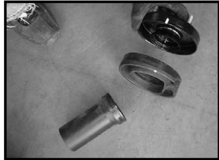
10. Locate (1) new front spacer. Install the new spacer into the upper bearing plate. **Special note: slight tapping of the spacer with a hammer will make installation easier.**
