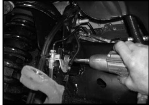
15. Working on the driver side re-install the tie rod ends back into the steering knuckle using the stock nut and torque to **70 ft lbs.** Repeat on passenger side.
