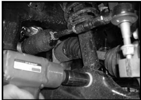
8. Working on the driver side, loosen but do not remove the (2) bolts holding the lower control arm to the vehicle. Repeat
