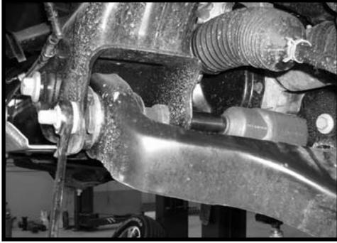
9. With both strut assemblies out of the vehicle it is time to install the new leveling spacers. Install these directly on top of the stock strut cap and secure them using the stock nuts. Torque to **35 ft lbs.**
