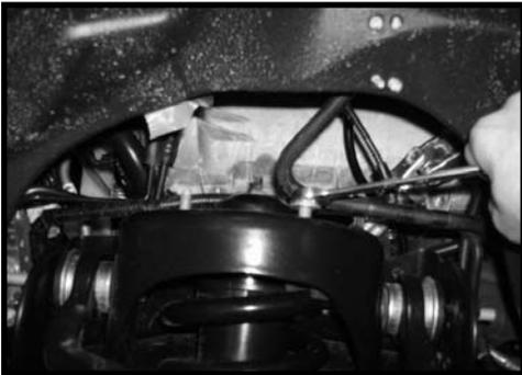
3. Working on the driver side, Loosen, but do not remove the upper ball joint nut. Repeat procedure on the passenger side.
