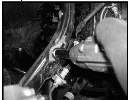
28. Locate the ABS mounting hardware. Working on the driver side, secure the ABS bracket to the upper control arm and secure using the hardware. Make sure to add some loctite
