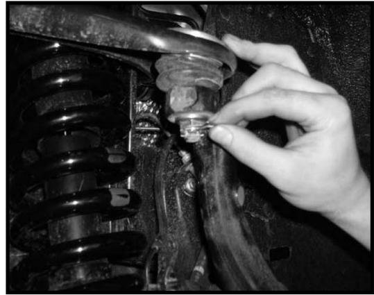
25. Locate the outer tie rod castle nut. Working on the driver side, install the outer tie rod the knuckle and secure using the castle nut. Make sure add some loctite and torque to **67 lbs.**
