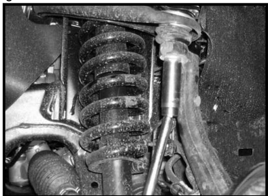
7. Working on the driver side, remove the cotter pin from the outer tie rod ball joint. Save the cotter pin for later re-installation. Repeat procedure on the passenger side.
