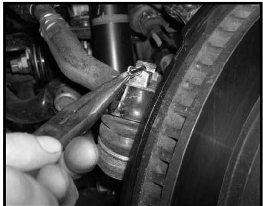
27. Locate the brake line mounting hardware. Working on the driver side, secure the brake line bracket to the knuckle and secure using the OE hardware. Make sure to add some loctite and torque to **12 lbs.**
