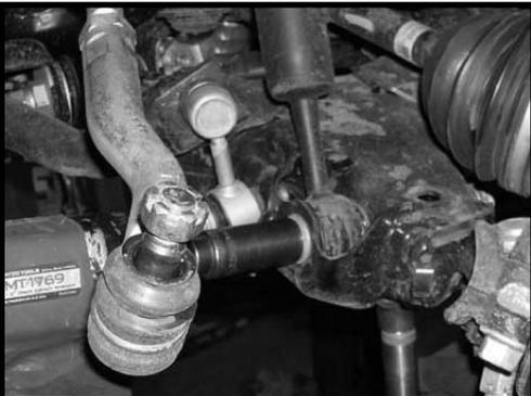
12. Working on the driver side, remove the sway bar end link hardware that connects the sway bar end link to the lower control arm. Save the hardware for later re-installation. Repeat procedure on the passenger side. Let the stock sway bar hang.
