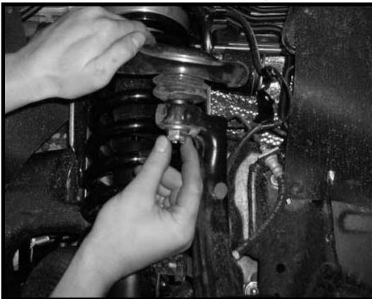
24. Locate the upper control arm cotter pin. Working on the driver side, install the cotter back into the upper control arm ball joint. **Special note: If the cotter pin can not be installed because the hole in the castle nut does not line up with the ball joint, DO NOT loosen the castle nut so that the cotter pin can fit, tighten the castle nut some more so that the cotter pin can be installed.**
