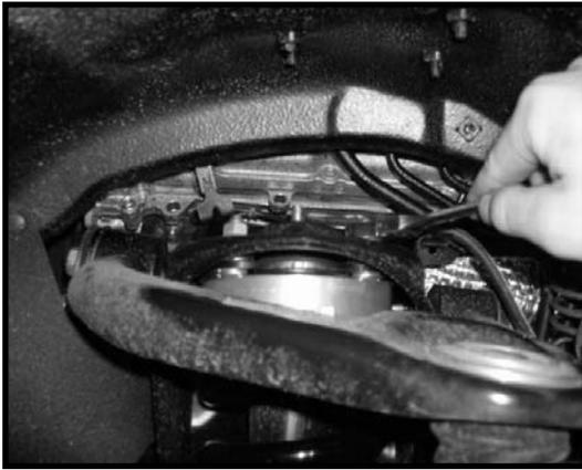
19. Locate the sway bar end link mounting hardware. Working on the driver side, secure the sway bar end link to the lower control arm using the OE hardware. Add some loctite and torque to **60 ft lbs.**
