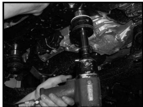
33. Locate the skid plate and the skid plate hardware. Install the skid plate into the OE location and secure using the hardware. Make sure to use loctite and torque all skid plate mounting hardware to **18 ft lbs.**
