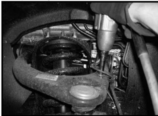
3. Working on the driver side, remove the hardware that connects the brake line bracket to the knuckle. Save the hardware for later re-installation. Repeat procedure in the passenger side.
