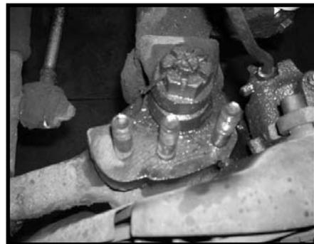
21. Locate the new steering arm. Install the new steering arm to the (3) stock studs. Install the (3) stock cone washers then using the (3) new 9/16" unitorque nuts that were packaged with the new steering arm, secure the new steering arm to the stock location. **Make sure to add some thread locker or loctite and torque to 115 ft lbs.**
