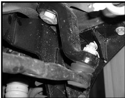
47. Locate the stock steering stabilizer hardware and the stock steering stabilizer. Install the stock steering stabilizer to the newly installed steering stabilizer bracket and secure using the stock hardware. Make sure to use thread locker or loctite and torque to **45 ft lbs.**
