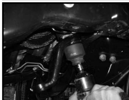
22. Locate the new track bar relocation bracket and the stock hardware. Install the new track bar to the stock location and secure using the stock hardware. **Special note: Make sure to install the leg of the new track bar re-**
