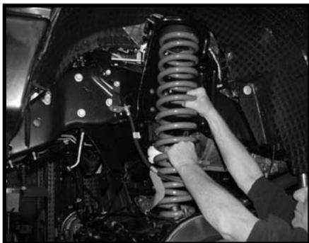
31. Locate the stock radius arm hardware that connected the stock radius arm to the stock radius arm bracket. Working on the driver side, install the stock radius arm to the new radius arm relocation bracket and secure using the stock hardware. Make sure to use thread locker or loctite and torque to **125 ft lbs.** Repeat procedure on the passenger side.
