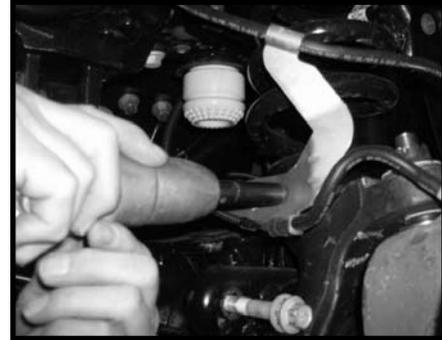
7. Working on the driver side, remove the stock brake line bracket from the stock location. Save the stock hardware. Repeat procedure on the passenger side. **Special note: On some vehicles, the stock brake line bracket is attached to the stock coil spring bucket.**
