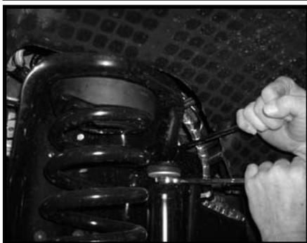
12. Carefully lower down on both hydraulic floor jacks at the same time allowing enough room for the stock coil springs to be removed. Working on the driver side, remove the stock coil spring from the stock location. Save the stock rubber isolator. The stock coil spring may be discarded. Repeat procedure on the passenger side.
