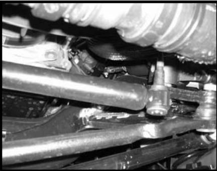
5. Move back to the stock hardware attaching the stock tie rod end to the stock pitman arm and remove. Set the stock hardware aside. Carefully break the stock taper and remove the stock tie rod from the stock pitman arm.
