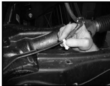
14. Working on the driver side, remove the stock hardware that connects the stock radius arm to the stock radius arm drop bracket. Save the stock hardware. Carefully lower down on both hydraulic floor jacks, this will allow the radius arm to come out of the stock location. Repeat procedure on the passenger side.
