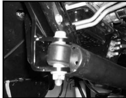
48. Locate the stock steering stabilizer hardware. Install the stock steering stabilizer to the stock location on the stock tie rod and secure using the stock hardware. Make sure to add some thread locker or loctite and torque to **45 ft lbs.**
