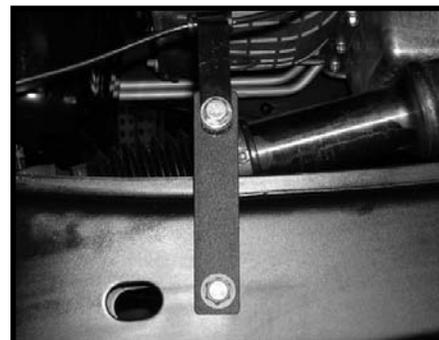
42. Working on the driver side, move back to the newly installed 9/16" x 1 1/2" bolts and hardware that is securing the new radius arm relocation bracket to the frame rail and add some thread locker or loctite. Torque all (7) bolts to **95 ft lbs.** **Special note: Torque the (3) bolts that hold the bracket to the bottom of the stock frame rail, then torque the (4) bolts that connect the bracket to the side of the stock frame rail.** Repeat procedure on the passenger side.
