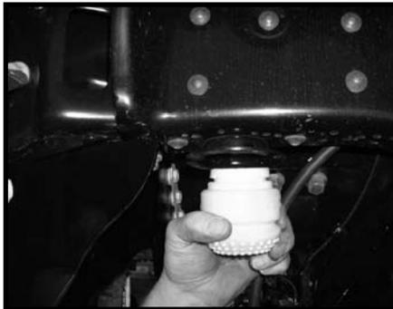
24. Working on the driver side, remove the stock bump stop cup from the bottom of the stock frame rail and save the stock bump stop cup and the stock hardware. Repeat procedure on the passenger side.
