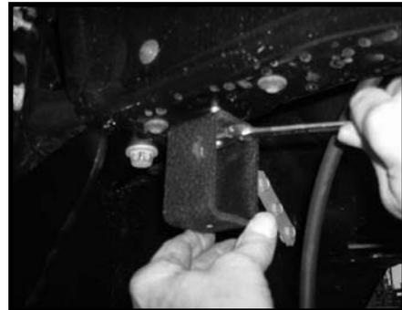
26. Locate the stock bump stop cups. Also, locate the (2) 5/16" x 1" bolts, (4) 1/4" USS flat washers and (2) 5/16" uni-torque nuts from hardware bag 24970NB. Working on the driver side, install the stock bump stop cup to the newly installed bump stop relocation bracket and secure using the new 5/16" x 1" bolts and hardware. Make sure to use thread locker or loctite and torque to **18 ft lbs.** Repeat procedure on the passenger side.
