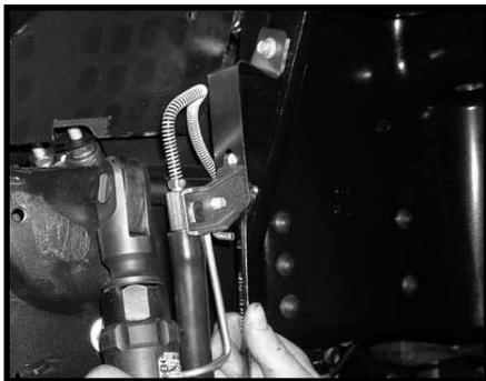
30. Locate the new coil springs. Also, locate the stock isolator. Working on the driver side, install the stock isolator on the new coil spring and install the new coil spring into the stock location. Carefully raise up on the hydraulic floor jack until the new coil springs seats properly into the stock upper and lower location. Repeat procedure on the passenger side.
