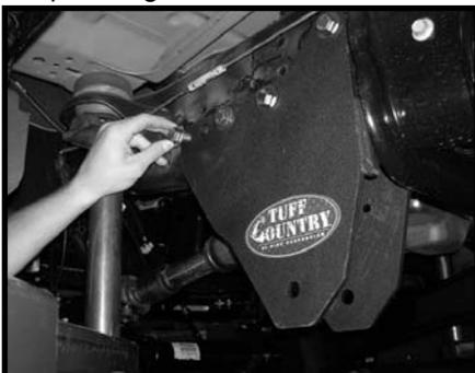
19. Working on the driver side, remove the stock hardware that attaches the stock track bar to the stock frame rail and cross member. **Special note: Heating up the bolts that connect the stock track bar to the bottom side of the stock frame rail will make removal easier. This will melt the thread locker.** Save the stock hardware for later re-installation. The stock track bar bracket may be discarded.
