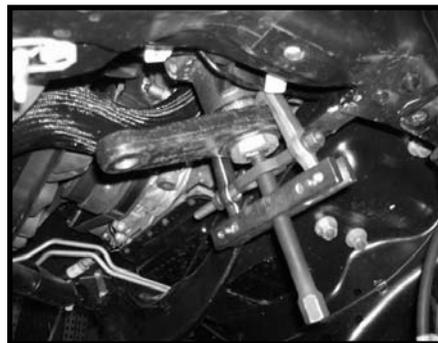
21. Locate the new pitman arm and the stock lock washer. Also, locate the new 30 mm jam nut from hardware bag 24970PL. Install the new pitman arm to the stock sector shaft and secure using the stock lock washer and new 30 mm jam nut. Make sure to use thread locker or lock tite and torque to **350 ft lbs.**
