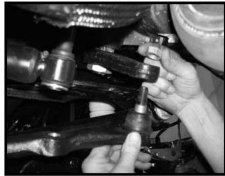
6. Working on the driver side, remove the stock lower brake line bracket from the stock front axle. Save the stock hardware. Repeat procedure on the passenger side.
