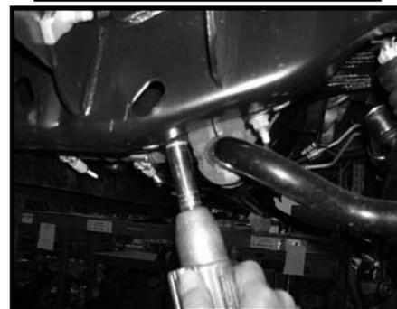
3. Working on the driver side, remove the stock cotter pin and re-taining nut that connects the stock tie rod to the stock pitman arm. Save the stock hardware. Loosen, but do not fully remove the stock nut that connects the stock tie rod to the stock pitman arm.
