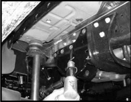
16. Working on the driver side, carefully drill out each hole where the rivets were located to a 9/16" hole. **Special note: Take special care not to drill into any wires or hoses that travel down the stock frame rail. Drill out (4) on the side of the stock frame rail and (3) on the bottom of the stock frame rail.** Repeat procedure on the passenger side.
