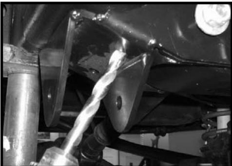
11. Locate (2) 1/2" x 1 1/2" bolts, (4) 7/16" USS flat washers and (2) 1/2" unitorque nuts from hardware bag 30940NB1. Working on the driver side, secure the new bracket to the bottom of the frame rail using the new 1/2" x 1 1/2" bolts and hardware. Make sure to use thread locker or loctite and torque to **55 ft lbs.**
