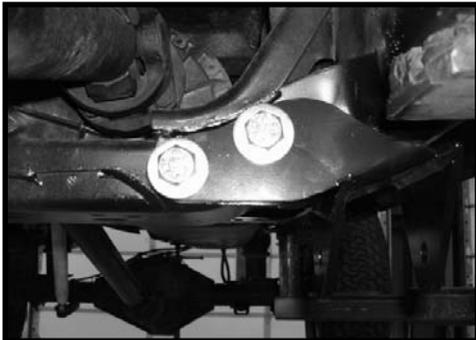
10. Working on the driver side, holding the new bracket up to the frame rail and carefully drill (2) 1/2" holes into the bottom of the frame rail using the holes in the new bracket as a guide.
