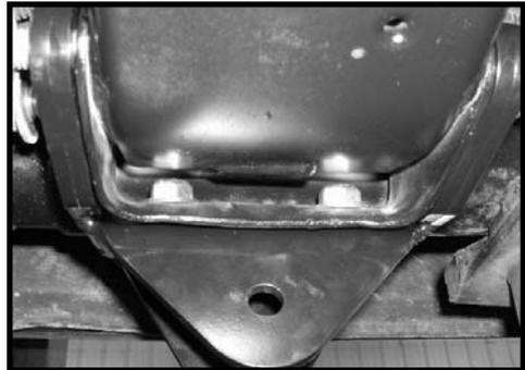
12. Working on the driver side, move back the new 9/16" x 8" bolts holding the legs of the new bracket to the transmission cross member and add some thread locker or loctite and torque to **85 ft lbs.** Now remove the hydraulic floor jacks from under the transmission cross member.
