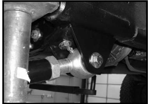
19. Locate the stock cam bolts and hardware. Install the new longer lower control arm to the axle mount and secure using cam bolts and hardware. For now, center the cam bolt and torque to **95 ft lbs.** Move back to the new mounting hardware that is securing the new longer lower control arm to the rear mount and add some thread locker or loctite and torque to **95 ft lbs.**
