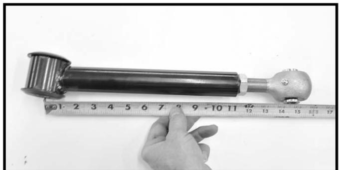
21. Working on the driver side, install the upper control arm to the front axle using the OE hardware. **Do not tighten at this point.** Repeat procedure on the passenger side.
