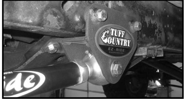
18. Locate the new driver and passenger side upper control arms and the smaller heim joints. Install the new heim joints into the ends of the new upper control arms. **Special note: Make sure to use a fair amount of anti-seize on the threads. If this is not done, the new long arm will not perform properly. Also, make sure that the sert fitting on the heim joint is in the upward position when installed in the vehicle.**
