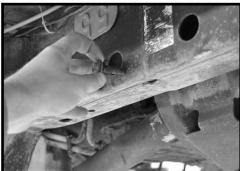
6. Working on the driver side and using the frame rail as a guide, carefully drill a 1/2" hole through the frame rail and the transfer case cross member. Make sure to drill out both the front and rear hole.
