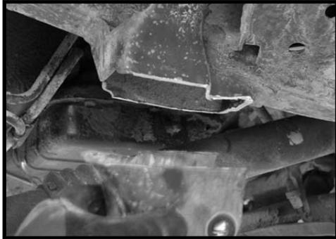
14. Locate the new driver and passenger side longer lower control arms and the larger heim joints. Install the new heim joints into the ends of the new longer lower control arms. **Special note: Make sure to use a fair amount of anti-seize on the threads. If this is not done, the new long arm will not perform properly.**
