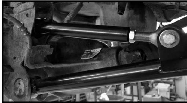
23. Working on the driver side, move back to the larger and smaller heim joints and tighten the locking nut on both. Repeat procedure on the passenger side.
