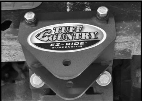
10. Working on the driver side move back to the new 1/2" hardware and add some loctite and torque all 4 bolts to **75 ft lbs.** Repeat procedure on the passenger side.
