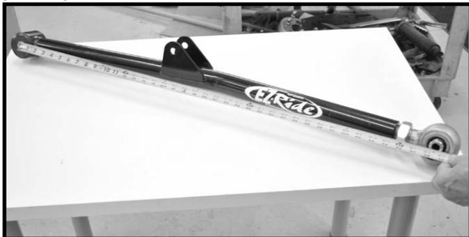
17. Locate (2) 9/16" x 4" bolts, (4) 1/2" USS flat washers and (2) 9/16" unitorque nuts from hardware bag 30945NB. Working on the driver side, install the new longer lower control arm to the newly installed frame bracket and secure using the new 9/16" x 4" bolt and hardware. **Do not tighten at this point.** Repeat procedure on the passenger side. **Special note: Also, make sure that the sert fitting on the**
