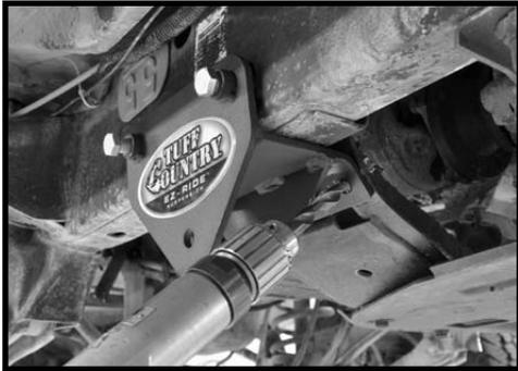
9. Locate (4) 1/2" x 1 1/2" bolts, (8) 7/16" USS flat washers and (4) 1/2" unitorque nuts from hardware bag 30945NB. Working on the driver side, secure the newly installed frame bracket to the transfer case cross member using the new 1/2" hardware. **Do not tighten at this point.** Repeat procedure on the passenger side.
