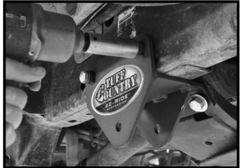
11. Working on the driver side, remove the upper and lower control arms. The control arms and frame mounting hardware may be discarded but save the axle mounting hardware. Repeat procedure on the passenger side.
