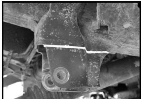
13. Working on the driver side carefully cut off the stock lower control arm rear bracket. **Special note: Make sure not to cut into the stock frame rail. Also, Tuff Country does not recommend using a torch when making this cut. Using a die grinder works best for this step.** Once the bracket has been cut away, clean and dress up any exposed metal. Repeat procedure on the passenger side.
