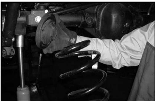
20. Locate the new rear coil spring spacers. Also, locate the stock driver and passenger side coil springs. Working on the driver side coil spring, place the new rear coil spring spacer on top of the stock coil spring and install the stock coil spring and new rear coil spring spacer back into the stock location. Repeat procedure on the passenger side. Carefully raise up on both hydraulic floor jacks until the stock coil springs and spacer seat properly into the upper and lower locations.
