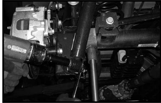
16. Working on the driver side, remove the lower mounting hardware that connects the stock sway bar end link to the stock lower bracket that is attached to the rear axle. Save the stock hardware for later re-installation. Repeat procedure on the passenger side. Let the stock sway bar hang.
