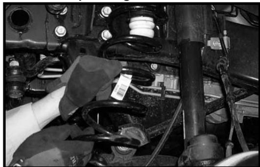
6. Locate the new front coil spring spacers. Working on the driver side, install the new coil spring spacer over the stock bump stop cup. Repeat procedure on the passenger side.
