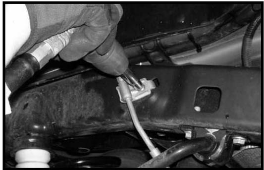
23. Locate the stock lower shock mounting hardware. Working on the driver side, install the stock shock into the stock lower mounting location and secure using the stock hardware. Make sure to use thread locker or loctite and torque to **65 ft lbs**. Repeat procedure on the passenger side.
