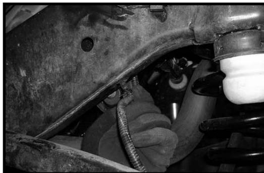
28. Locate the stock brake line hardware. Working on the driver side, re-install the stock brake line bracket to the side of the stock frame rail using the stock hardware. Repeat procedure on the passenger side.
