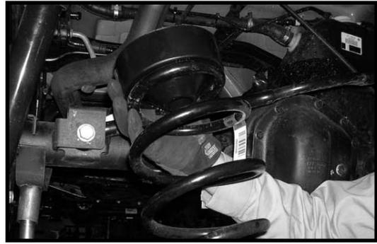
21. Working on the driver side, carefully push the stock ABS clip back into the bottom side of the stock frame rail. Repeat procedure on the passenger side. **Special note: Take care not to damage the stock ABS clip during installation.**
