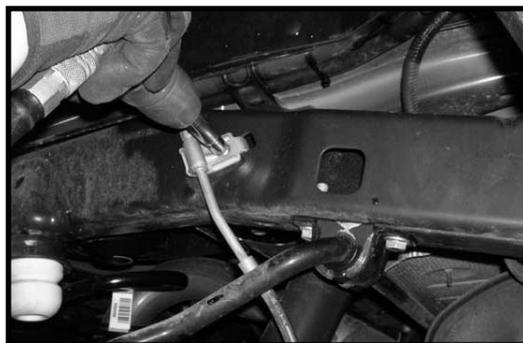
29. Locate the stock lower shock mounting hardware. Working on the driver side, install the stock shock into the stock lower mounting location and secure using the stock hardware. Make sure to use thread locker or loctite and torque to **65 ft lbs.** Repeat procedure on the passenger side.
