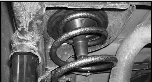
21. Locate (2) 3/8" x 1" bolts, (2) 3/8" lock washers, (2) 3/8" flange nuts from hardware bag 43000NB. Also, locate (2) rear spring retaining washers & (1) 43000-04 nut bracket from hardware bag 43000NB1 Working on the driver side, attach the new rear spring retaining washer on the bottom inside of the new coil and secure using the new 3/8" x 1" bolt and hardware and nut bracket. Make sure to use loctite and torque to **18 ft lbs.** Repeat procedure on the passenger side.
