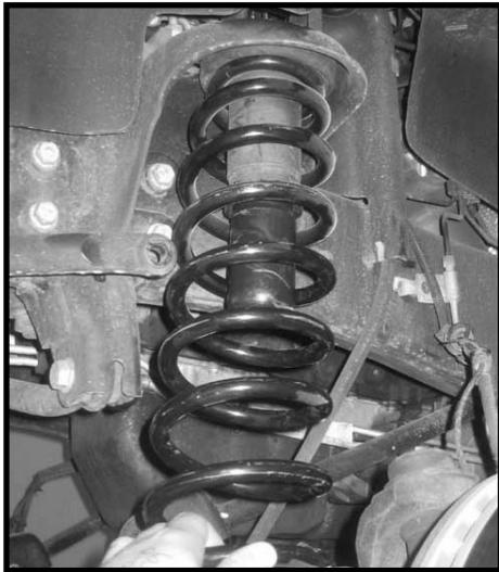
8. Locate the new front shocks. **Special note: New longer front shocks are needed after this suspension system has been installed and the shocks need to be ordered as a separate part #. If you have not already ordered your shocks, please feel free to contact Tuff Country or your local Tuff Country dealer and order your new shocks. Tuff Country recommends installing a 26" fully extended shock in the front.**
