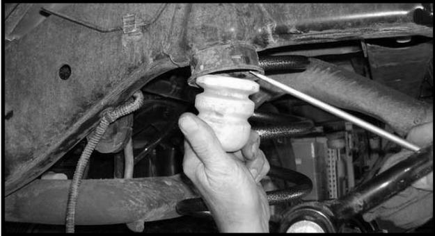
16. Locate the new rear bump stops. Working on the driver side, install the new rear bump stop into the stock location. Repeat procedure on the passenger side. **Special note: using some lithium base grease will help make installation easier.**
