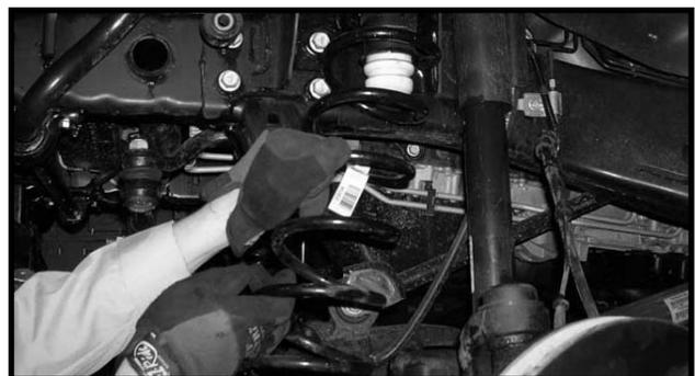
6. Locate the new front bump stops. Working on the driver side, remove and discard the OE bump stop. Install the new extended bump stop into the stock location. Repeat procedure on the on the passenger side.
