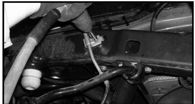
14. Working on the driver side, carefully remove the ABS line clip from the bottom of the frame rail. Repeat procedure on the passenger side.
