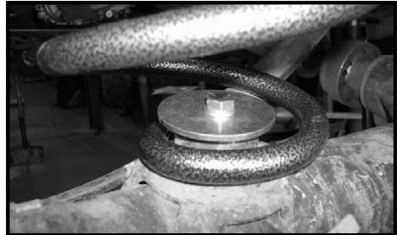
22. Locate the new track bar relocation bracket. Locate (1) S10065 sleeve from hardware bag 43000NB1. Also, locate (1) 9/16" x 3 1/2" bolt, (2) 1/2" USS flat washers and (1) 9/16" unitorque nut from hardware bag 43000NB. Install the new track bar bracket into the OE location and secure using the new hardware into the OE location. **Do not tighten at this point.**
