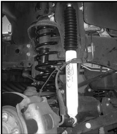
9. Working on the driver side, install the rear sway bar end link into the front location using the OE lower hardware and the stock upper hardware. Make sure to use loctite and torque the lower hardware to **55 ft lbs** and the upper hardware to **55 ft lbs.** Repeat procedure on the passenger side.
