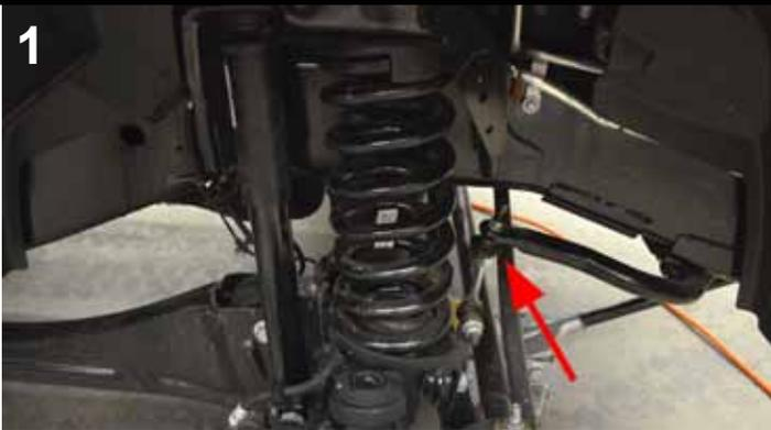
Remove wheels and tires. Raise the truck with a jack and place on jack stands at the chassis. Disconnect sway bar link at the sway bar on both sides.
