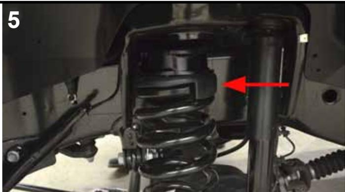
Install coil springs and Spacer back into vehicle, making sure coil spring is positioned as shown in image. Raise the axle while guiding coil springs into place.
