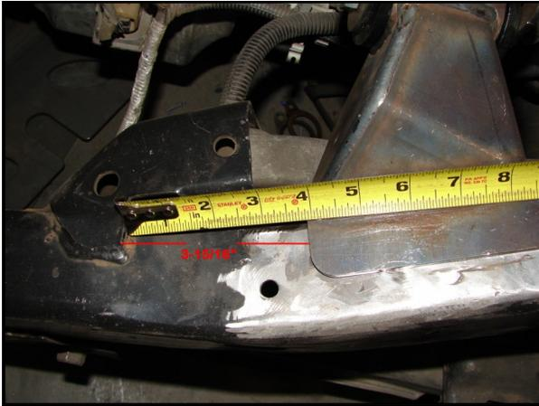
Passenger side : Measure from the Upper Control arm bracket to the back side of the JM700 Mount. This measurement should be **3-15/16"**
