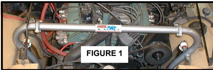
SH200 installed on a 1978 Jeep® CJ-7 with AMC V-8 and Power steering. Note how the cross-over tube sits in front of the power steering pump.
