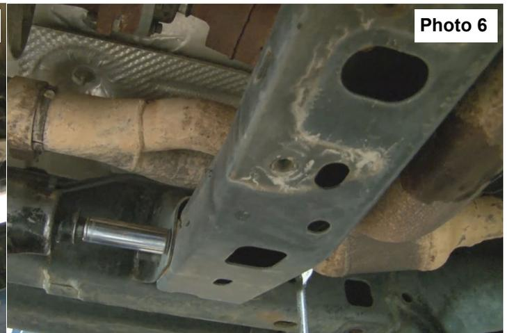
7. Place the new cross member into the frame pockets and tighten using factory bolts and a 18mm socket and wrench.
