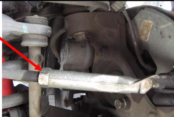
**2 )** Next remove the tie rod ball joint 22mm nut ( counter clockwise ) Save it you will re-install it later.
