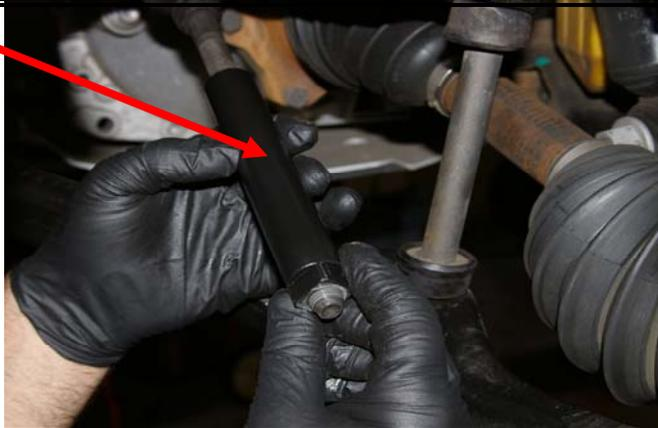
5 ) While holding the support tube with one hand making sure not to move it and lose the location, install your factory tie rod steering ball joint end ( clockwise ) until it meets up with the ReadyLift support tube. Lock them together hand tight while positioning the ball joint threaded end pointed up to fit back into the spindle.
