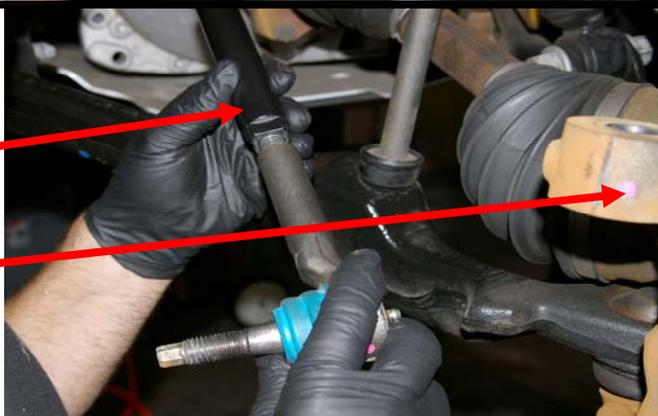
6 ) install the ball joint into the spindle and thread on the Factory 22mm nut flat surface down and torque to factory specs. You may need a small open end wrench to hold the ball joint shaft from spinning while tightening the 22mm nut.
